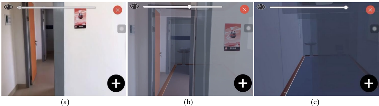
Fig. 2. Examples of alpha channel, where: (a) alpha channel at 0%, where only the real world is visualized; (b) alpha channel approximately at 50%, which shows a mixed world between the real and the virtual; (c) alpha channel at 100%, which shows the virtual world
