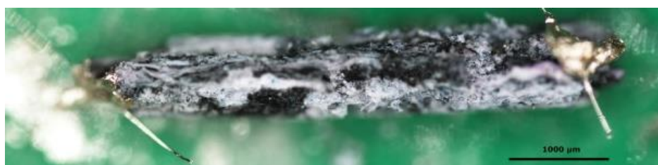
Figure S13. Detail of the LDH@CNT hollow composite structure mounted on the electrical measurement set-up.
