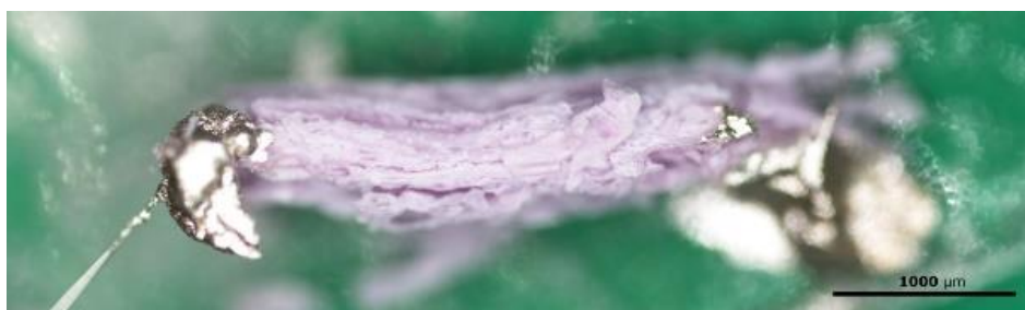
Figure S12. Detail of the bare ZnCr LDH hollow structure mounted on the electrical measurement set-up.
