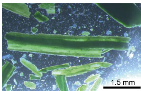
Figure S15. Optical micrograph of \alpha -NiCo LH hollow structures obtained at TFR 2100 \mu\text{L}/\text{min} and FRR 0.3, showing the intense green colour of the material.
