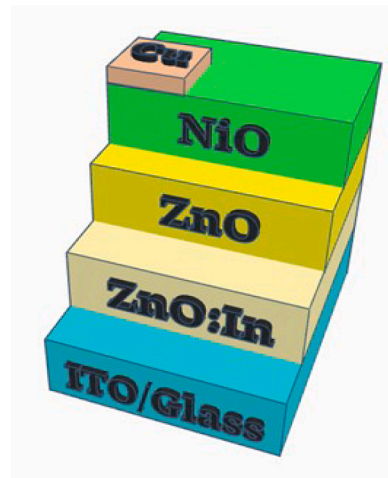
Fig. 1. Schematic representation of a Glass/ITO/ZnO:In/ZnO/NiO/Cu multilayer structure (a).
