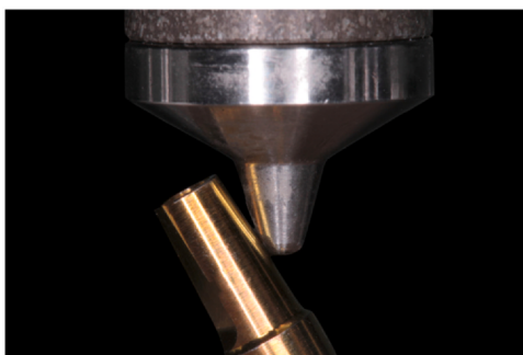
Figure 2. Dynamic mechanical load test of implant-prosthetic abutments.
