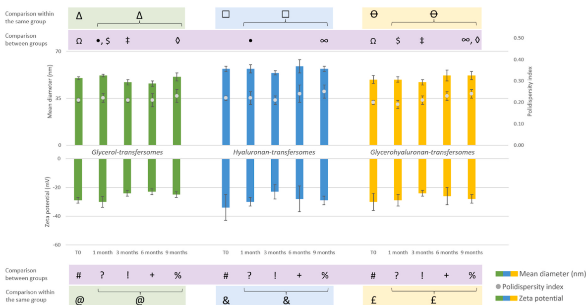
Fig. 2. Stability over time evaluated by measuring mean diameter (upper panel, bars), polydispersity index (upper panel, dots), and zeta potential (lower panel, bars) of glycerol-transfersomes (green), hyaluronan-transfersomes (blue) and glycerohyaluronan-transfersomes (orange). The same symbols (Δ, □, Θ, Ω, •, $, ‡, ∞, #, ?, !, +, %, @, & and £) indicate values that are not statistically different ( p > 0.05 ) from the values at the initial time (light green, blue and orange) or among the different groups (cross-comparison) at the same time point (violet). Different symbols indicate significant differences ( p < 0.05 ). Mean values \pm standard deviations, obtained from at least 3 measurements, are reported. (For interpretation of the references to color in this figure legend, the reader is referred to the Web version of this article.)
