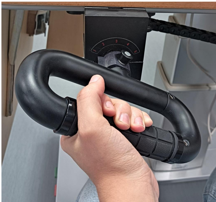
Figure A-1. Handle of the measuring device, with marks for 60° (60SUP and 60PRO), 30° (30SUP and 30PRO) and 0° (NEU) postures represented by numbers 1 to 5.
