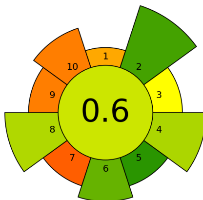
Figure 4.9. AGREEprep pictogram of the proposed method. (1-Sample preparation placement; 2-Hazardous materials; 3-Sustainability and renewability of materials; 4-Waste; 5-Size economy of the sample; 6-Sample throughput; 7-Integration and automation; 8-Energy consumption; 9-Post sample preparation configuration for analysis; 10-Operator's safety).
