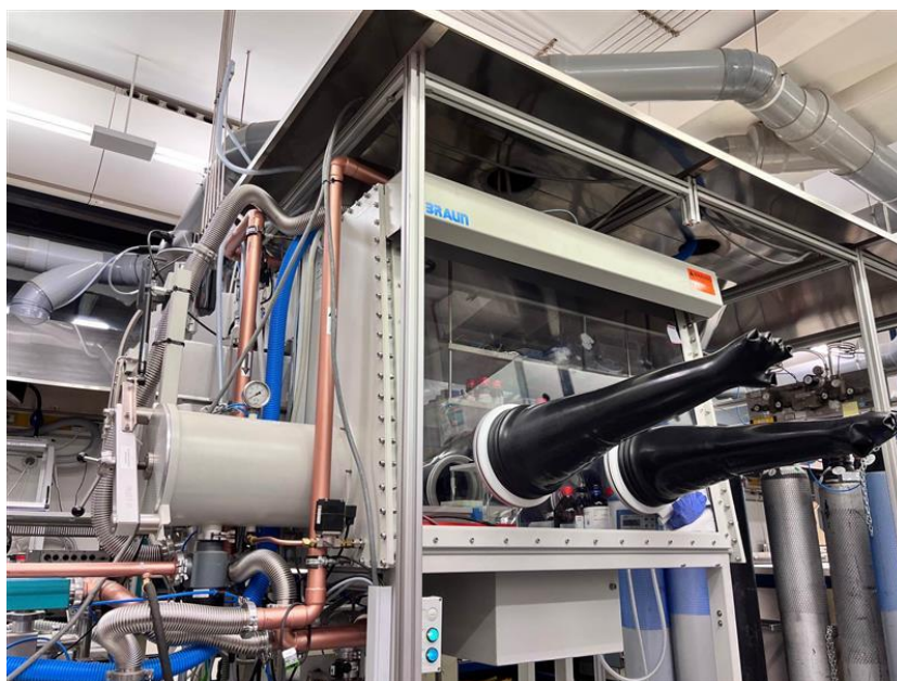
Figure 22. ABX 3 Lab glovebox set-up for the fabrication of MHPs. The evaporator is located right behind the main antechamber (left side of the picture).
