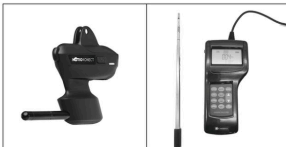
Figure 2. Notio on the left and hot-wire anemometer Kanomax Anemomaster 6036-CE on the right. Original images from the manufacturer manuals with permission.
