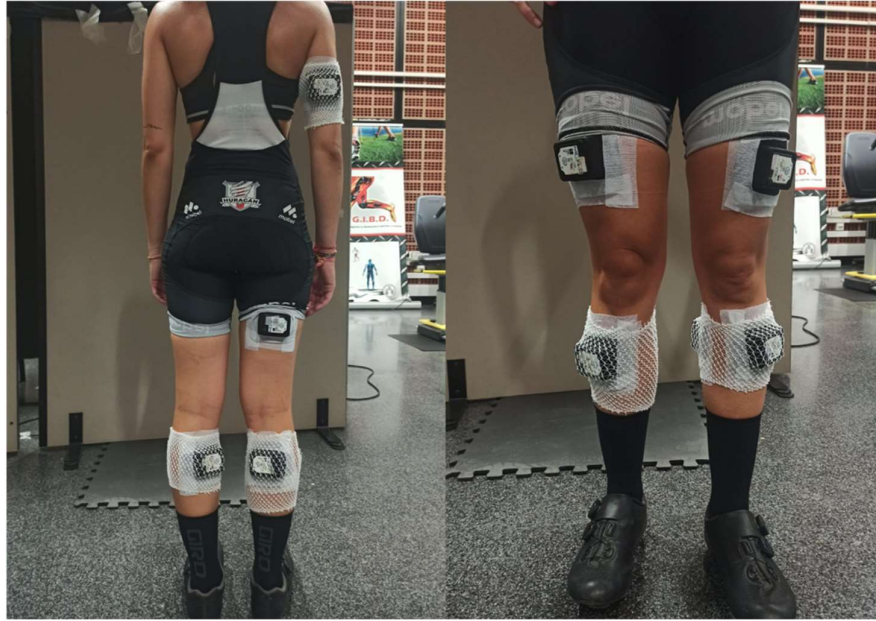
Figure 2.4. Location of the Moxy Monitor devices in graded exercise and 8-min Functional Threshold Power estimation test.
