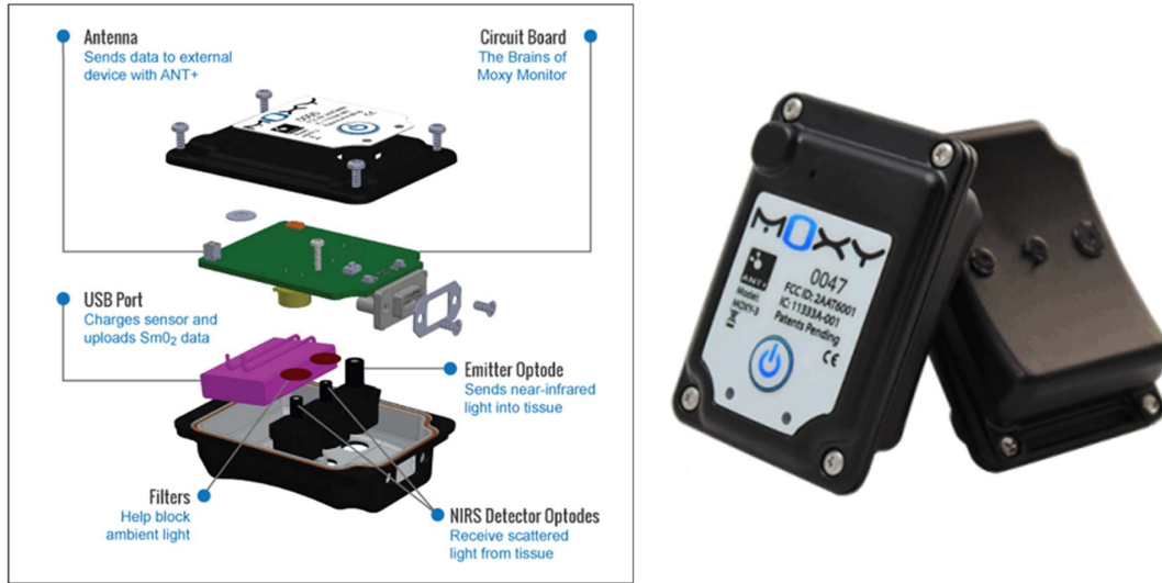
Figure 2.3. Near Infrared spectroscopy portable. Moxy Monitor sensor used in experimental study.
