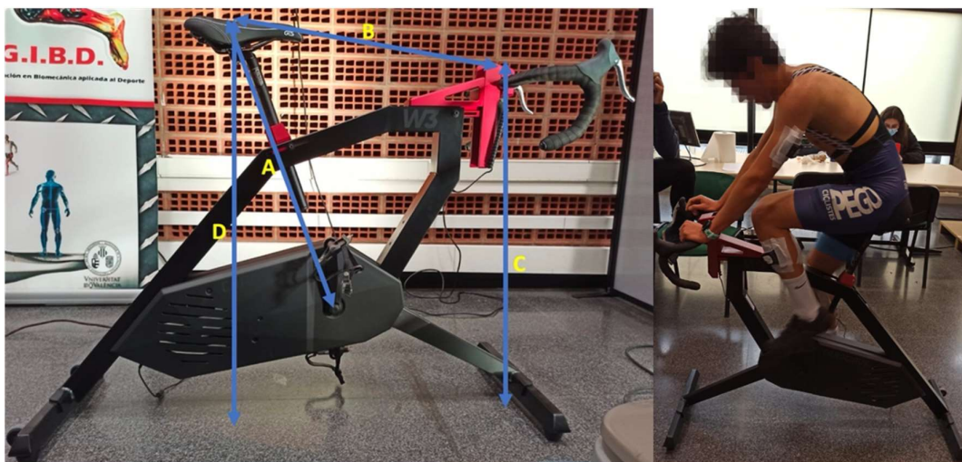
Figure 2.1. Cycle ergometer used and bike measurements. (A) Distance from bottom bracket to saddle center; (B) Distance from saddle center to intersection between stem and handlebars;
