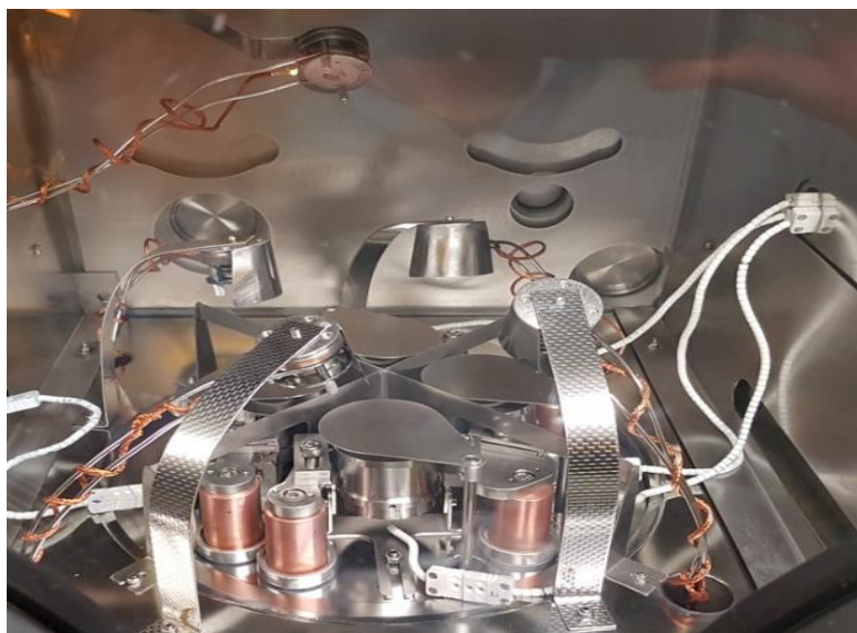
Figure 2-2: Inside one of the vacuum chambers used for vacuum sublimation in the current thesis.
