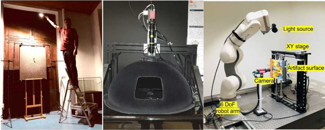
Figure 1: some examples of RTI implementation. Handhel (left), Dome-based (middle) and Robotic-arm based ((right)
