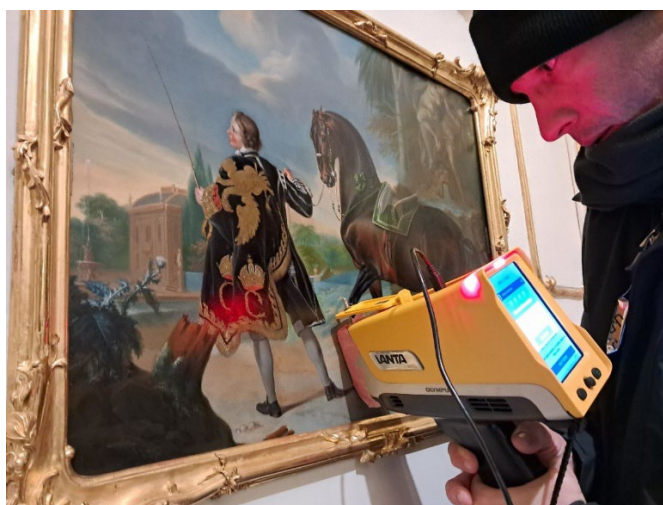
Figure 3. Running pXRF analysis to identify the elemental profile of pigments in an artwork at Schönbrunn Palace (Vienna Austria) under the framework of ChemiNova project ( https://cheminova.eu/ ).
