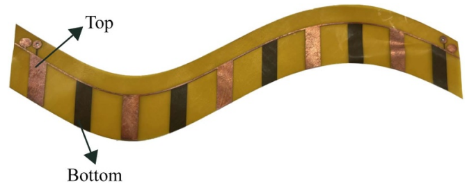
Figure 2. View of the capacitive sensor deployed to be adapted to the bPMMA applicator. The sensor geometry follows the perimeter of the ellipsoidal end of the applicator.
