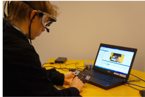
Fig. 1. Configuration of experiment. Participant played a mobile game while their eye movements were being recorded using Dikablis eye tracker. Two markers were attached on the smartphone as a reference for eye tracking data analysis.
