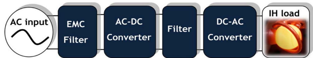
Figure 2. Schematic diagram of an IH generator [1].
