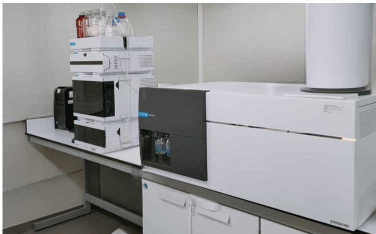
Figure 28. Agilent 6546 LC/QTOF equipped with an ESI interface. The analytical separation was carried out using an Agilent 1290 Infinity II series UHPLC.
