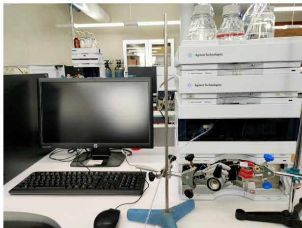
Figure 26. Agilent 1260 infinity series capillary LC equipped with a Rheodyne 7721-I injection valve for sample injection.
