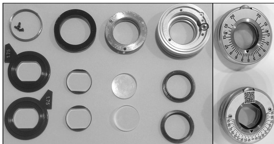
FIGURE 1 Exploded view of the built \pm 1.75 D Stokes lens with variable power. The top row on the left side of the picture shows an exploded view of the elements comprising the Risley mount, from left to right: screws to fix the mount to the phoropter, lock washer, black rotating ring, metallic cap to close the mount and the holder main body (with the toothed gear in place). The middle row shows, from left to right: a regular -1.75 D cylinder lens from a trial case, the same lens out of its frame and cut to the size of the mount, one of the prisms forming the Risley prism (that will be stored and not used in this work) and one of the gear wheels previously occupied by a prism that will now house the -1.75 D cylinder lens. The bottom row shows, from left to right: a regular +1.75 D cylinder lens from a trial case, the same lens out of its frame and cut to the size of the mount, one of the prisms forming the Risley prism (that will be stored and not used in this work), and one of the gear wheels previously occupied by a prism that will now house the +1.75 D cylinder lens. The right side of the picture shows a regular Risley prism inside its holder just removed from the phoropter (top) and the final result after conversion into a Stokes lens (bottom; notice the angular dial attached to the mount for direct determination of the rotation angle and the QR code).
