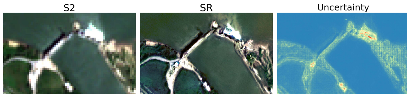
Fig. 11. Example of the uncertainty product delivered with the SR result, based on a real S2 input. The uncertainty values are visualized on a scale from blue (low) to red (high), stretched to the min-max range of the standard deviation.
