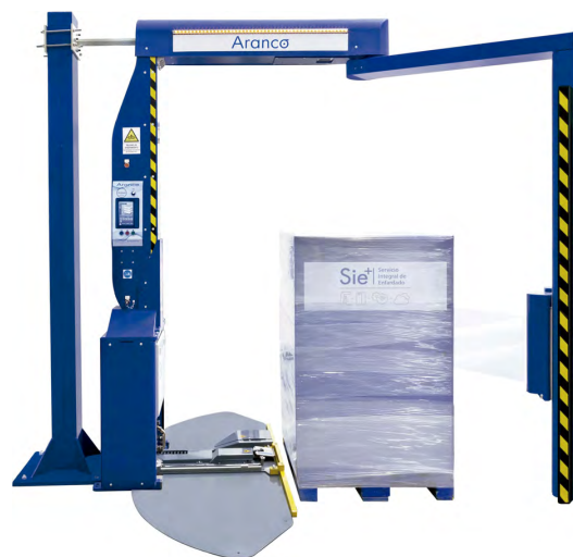
Figure 1. Automatic fixed wrapping machine F-2200 (Aranco, Valencia, Spain). Source: https://www.aranco.com/en/services/sie-wrappers/fixed-wrapping-machine-f-2200 (accessed on 16 December 2024).
