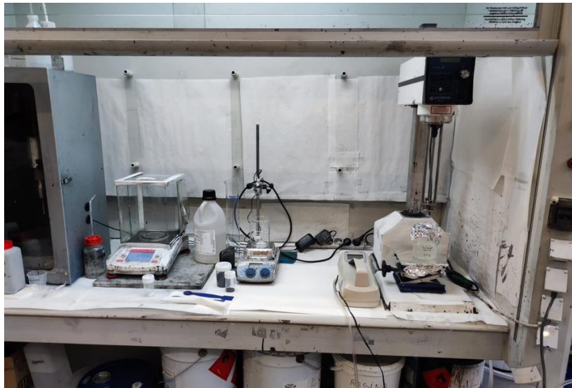
Figure 2: LEV (fume hood) used for the MW-assisted exfoliation of graphite to graphene.
