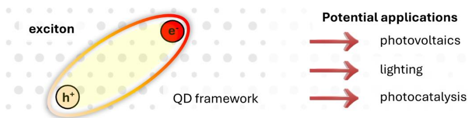
Figure 1.2. Representation of an exciton in a quantum dot framework after light interaction, and its potential application in the field of photovoltaics, lighting, and photocatalysis.
