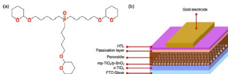
Figure 1. (a) Molecular structure of THPPO and (b) device structure of n-i-p PSCs employing fluorine-doped tin oxide (FTO), compact TiO 2 (c-TiO 2 ), mesoporous TiO 2 (mp-TiO 2 ), SnO 2 , perovskite, THPPO as a passivation layer, HTL, and gold electrode.
