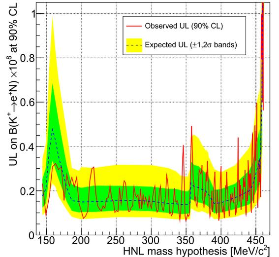
**Fig. 5.** The obtained upper limits at 90% CL of  $\mathcal{B}(K^+ \rightarrow e^+ N)$  and the expected  $\pm 1\sigma$  and  $\pm 2\sigma$  bands in the background-only hypothesis for each HNL mass value considered.
