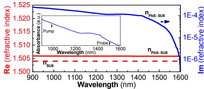
Fig. 2. Real (red solid line) and imaginary (blue solid line) parts of the PbS-SU8 (*ff* = 0.01) refractive index and real (red dashed line) part of the SU8 refractive index. The inset shows the absorption spectra of the PbS-SU8 QDs at pump (980 nm) and probe (1550 nm) wavelengths.
