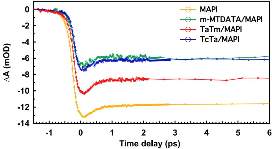
**Figure 4.** Time-resolved transient absorption dynamics for neat MAPI and the perovskite/HTM double layers, excited at 600 nm (at constant excitation density of  $1.4 \cdot 10^{17} \text{ cm}^{-3}$ ) and probed at the perovskite maximum ground state bleaching band.
