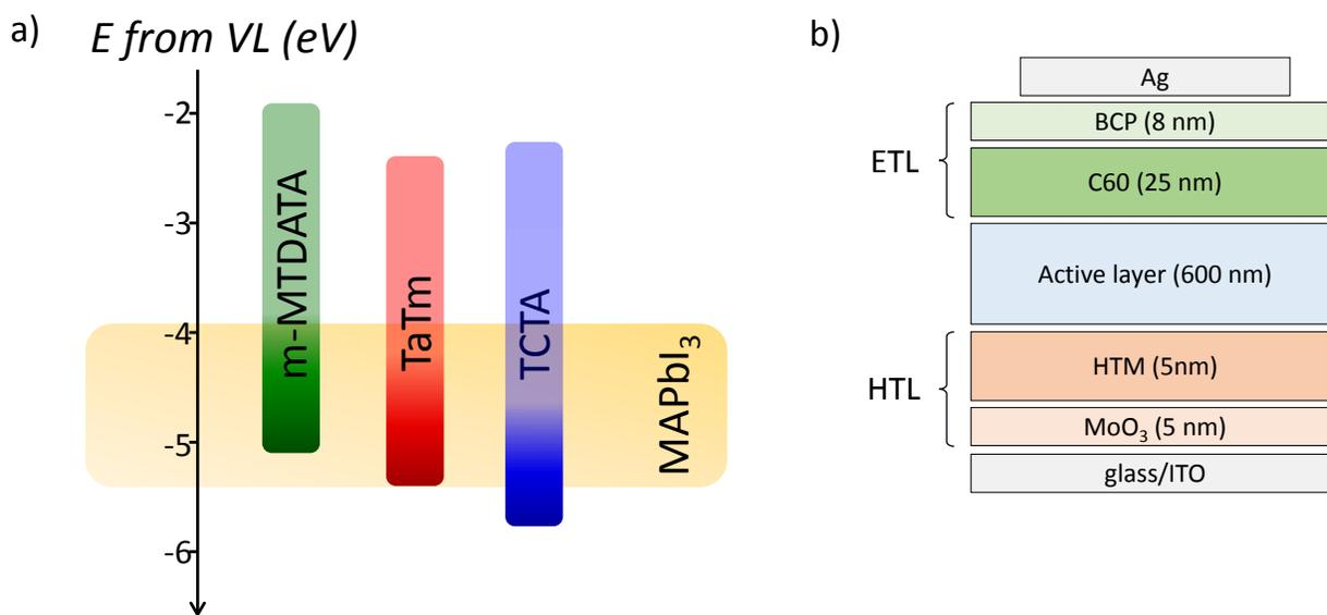
**Figure 1.** a) Energy diagram of different HTMs with respect to MAPbI<sub>3</sub>. The energy values of the HOMOs were determined by photoemission spectroscopy in air (PESA) (see supporting Information Figure S1). b) Scheme of completed stack with different HTMs.
