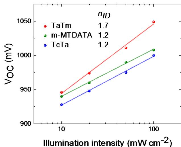
**Figure 3.** Light intensity dependent  $V_{oc}$  and extracted ideality factors for perovskite solar cells with different HTMs.
