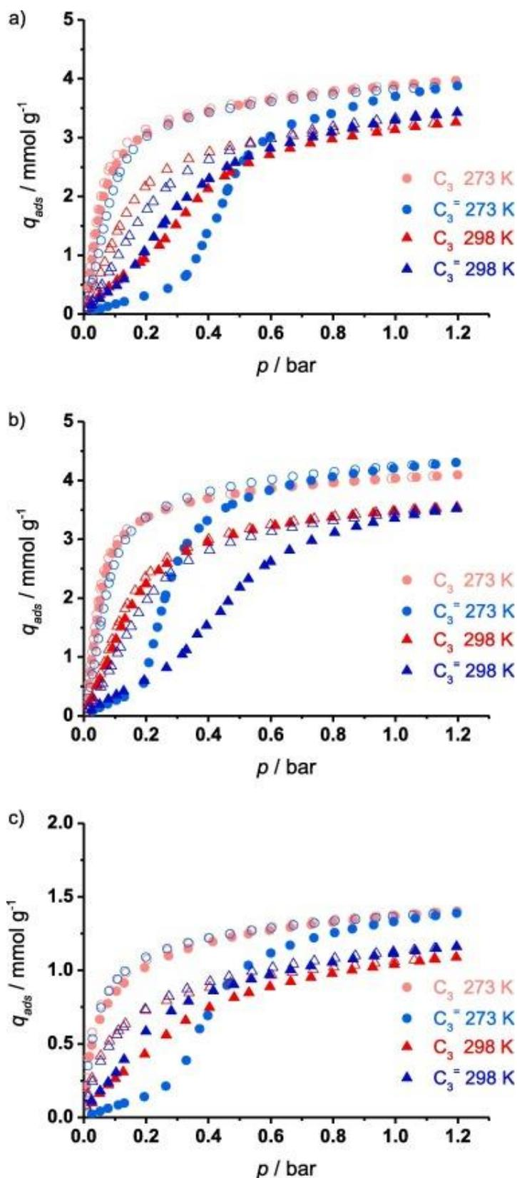
Fig. 3. Low pressure adsorption/desorption isotherms (volumetric measurement) for propane (red) and propylene (blue) at 273 K (spheres) and 298 K (triangles), on: (a) ZIF-8, (b) ZIF-67, and (c) MUV-3. Solid symbols for adsorption and open ones for desorption.
