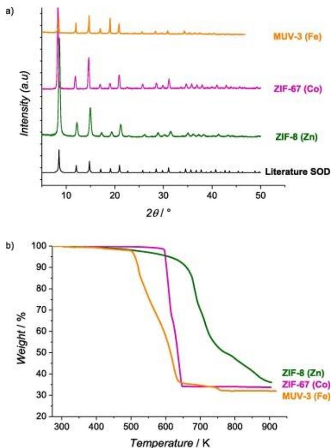
Fig. 1. ZIF-SOD characterization by (a) XRD ( $\lambda = 1.788970 \text{ \AA}$ ); and (b) TGA in air at  $5 \text{ K min}^{-1}$ .
