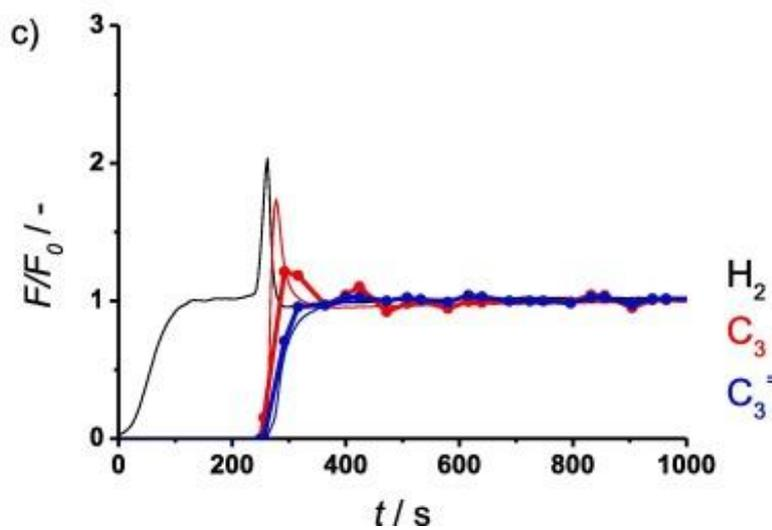
Fig. 6. Breakthrough normalized exit flowrates vs time for propylene rich feed ( $C_3:C_3^=:H_2 = 0.5:3.5:1$ ) at 298 K and 2 bara on (a) ZIF-8, (b) ZIF-67, and (c) MUV-3. CGC analysis (lines, symbols) over MS analysis (lines).
