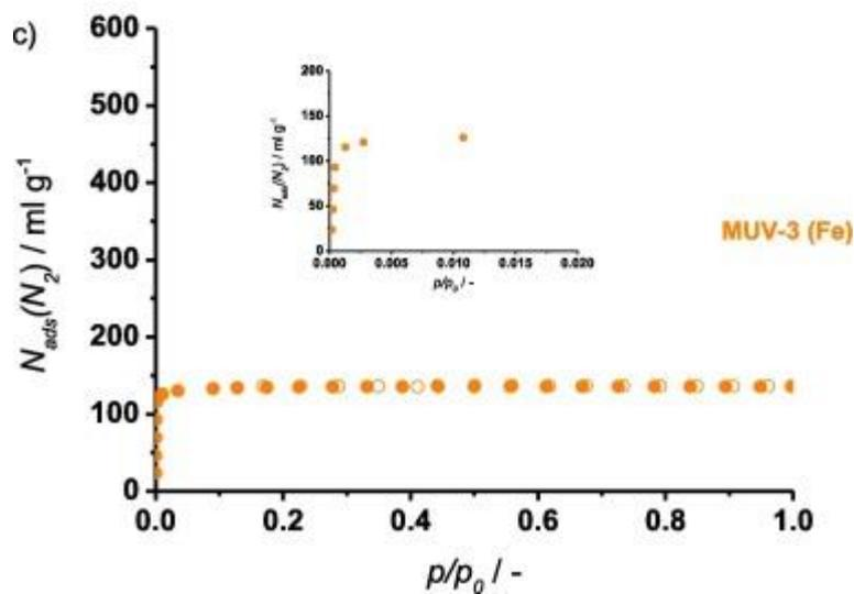
Fig. 2. Low pressure adsorption/desorption isotherms (volumetric measurement) for nitrogen at 77 K, on: (a) ZIF-8, (b) ZIF-67, and (c) MUV-3. Solid symbols for adsorption and open ones for desorption.
