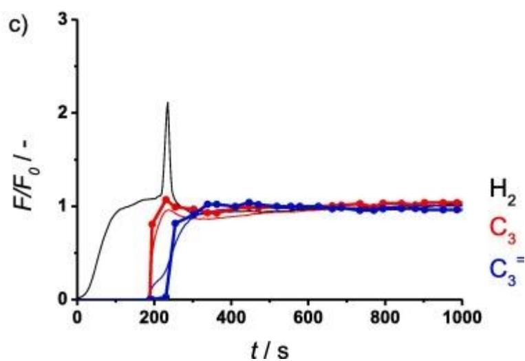
Fig. 5. Breakthrough normalized exit flowrates vs time for propane rich feed ( $C_3:C_3^-:H_2 = 3.5:0.5:1$ ) at 298 K and 2 bara on (a) ZIF-8, (b) ZIF-67, and (c) MUV-3. CGC analysis (lines, symbols) over MS analysis (lines).
