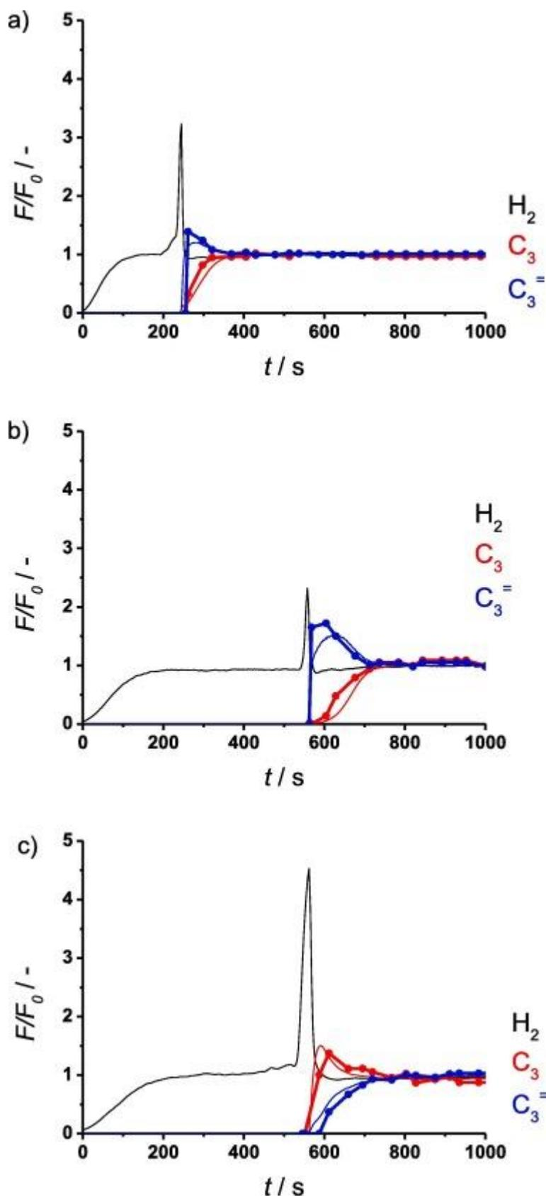
Fig. 4. Breakthrough normalized exit flowrates vs time for equimolar propane/propylene feed ( $C_3:C_3=:H_2 = 3.5:3.5:1$ ) at 298 K and 2 bara on (a) ZIF-8, (b) ZIF-67, and (c) MUV-3. CGC analysis (lines and symbols) over MS analysis (lines).
