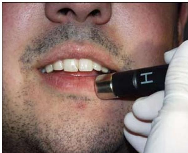
**Fig. 1.** Lip hydration measurement using Corneometer 825® (Courage & Khazaka Electronic GmbH, Cologne, Germany). To carry out the measurement, the sensor head is held at right angles to the lower lip, applying only the pressure exerted by the spring in the probe head.
