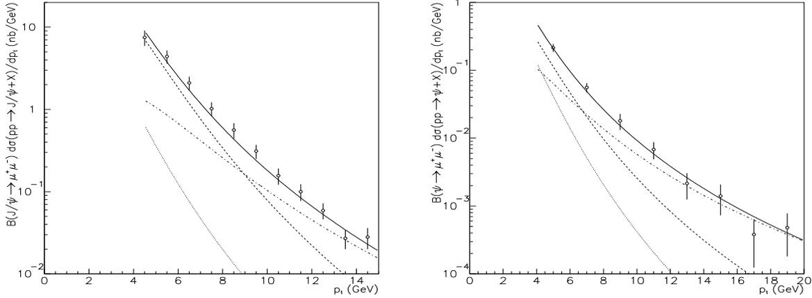
Figure 2: Two-parameter fits to the experimental Tevatron data using CSM + COM, where initial- and final-state radiation were incorporated via PYTHIA generation. a) (left)  $J/\psi$  and b) (right)  $\psi'$  production. The different contributions are shown separately i) dotted line: CSM, ii) dashed line:  $^1S_0^{(8)} + ^3P_J^{(8)}$ , iii) dot-dashed line:  $^3S_1^{(8)}$ , iv) solid line: all contributions.
