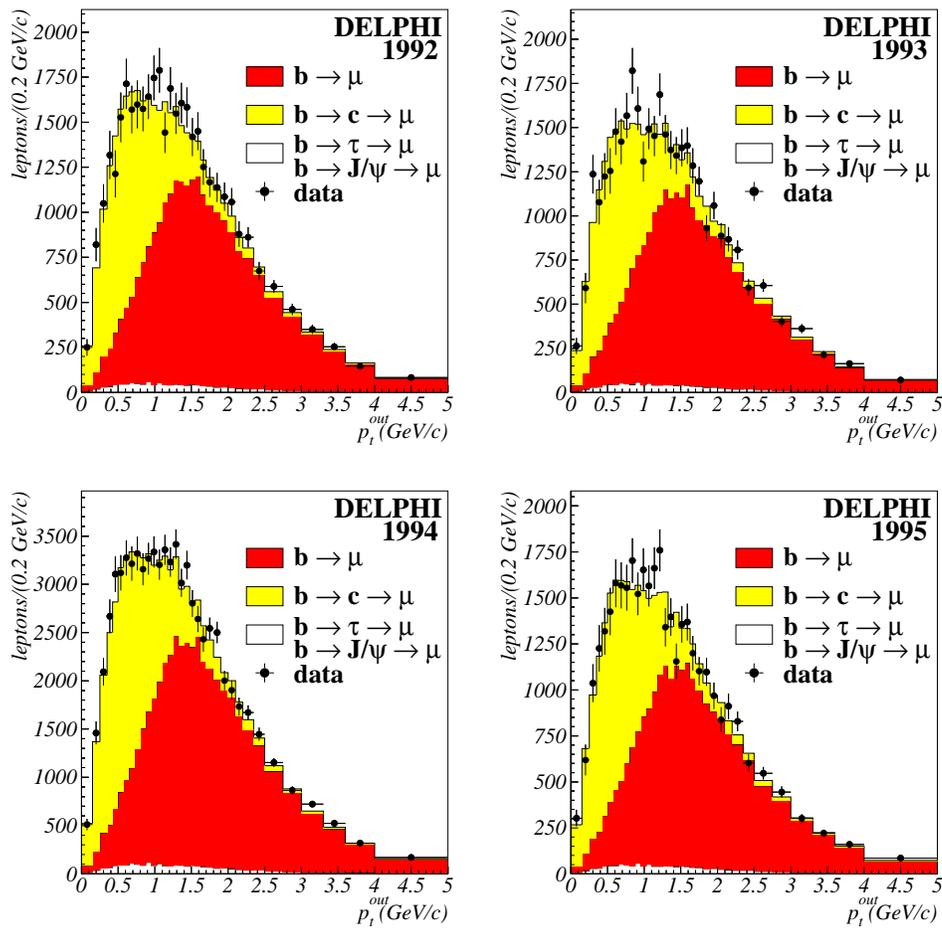
Figure 5: Comparison of the  $p_t^{out}$  distributions of prompt muons for the  $b$  flavour in real data (dots) with the distributions obtained using the semileptonic branching fractions (histograms). The contributions of different processes are displayed.
