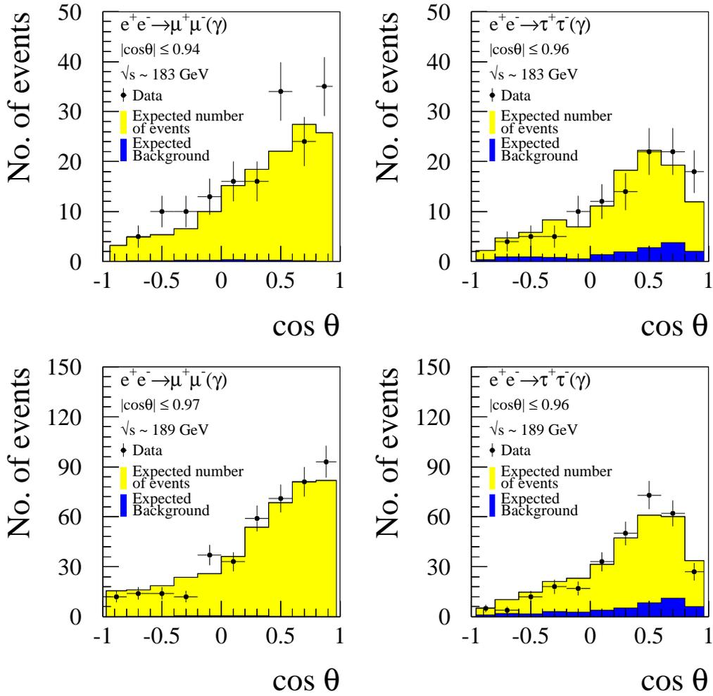
Figure 2: The numbers of events observed as a function of  $\cos \theta$  for  $\mu^+\mu^-$  and  $\tau^+\tau^-$  final states at centre-of-mass energies of  $\sim 183$  and  $189$  GeV. The points stand for the data and the histograms represent the signal and background. The expected signals are simulated with the KORALZ [11] generator scaled to the ZFITTER [12] predictions and normalised to the luminosities of the data sets analysed.
