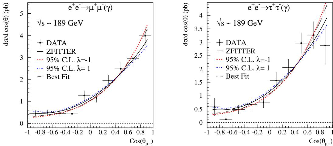
Figure 7: Fits to angular distributions for  $\mu^+\mu^-$  and  $\tau^+\tau^-$  final states, for models which include gravity in extra dimensions. The dashed fitted curves correspond to  $\epsilon = -8.39 \text{ TeV}^{-4}$ , the *best fit* to all data. The data are compared to the Standard Model predictions of ZFITTER and to the differential cross-sections predicted at 95% C.L. for  $\lambda = \pm 1$ .
