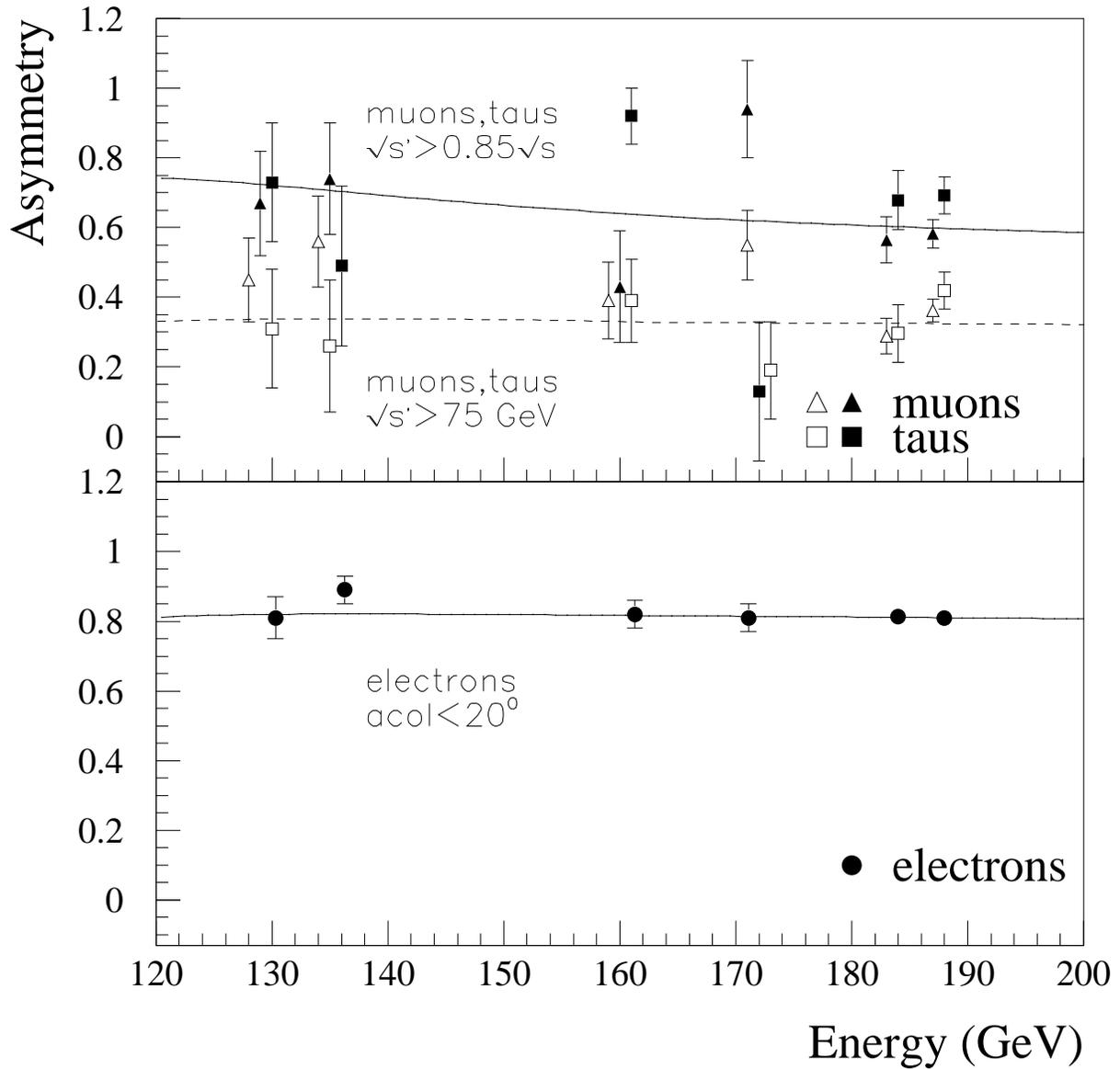
Figure 4: The forward-backward charge asymmetries in the reactions  $e^+e^- \rightarrow \mu^+\mu^-(\gamma)$ ,  $\tau^+\tau^-(\gamma)$  and  $e^+e^-(\gamma)$  measured at energies ranging from 130 to 189 GeV. The curves show the SM prediction of the TOPAZ0 program [13] for electron-positron final states and ZFITTER program [12] for the other final states. Solid points and solid lines represent the *non-radiative* selections, open points and dashed lines represent the *inclusive* selections.
