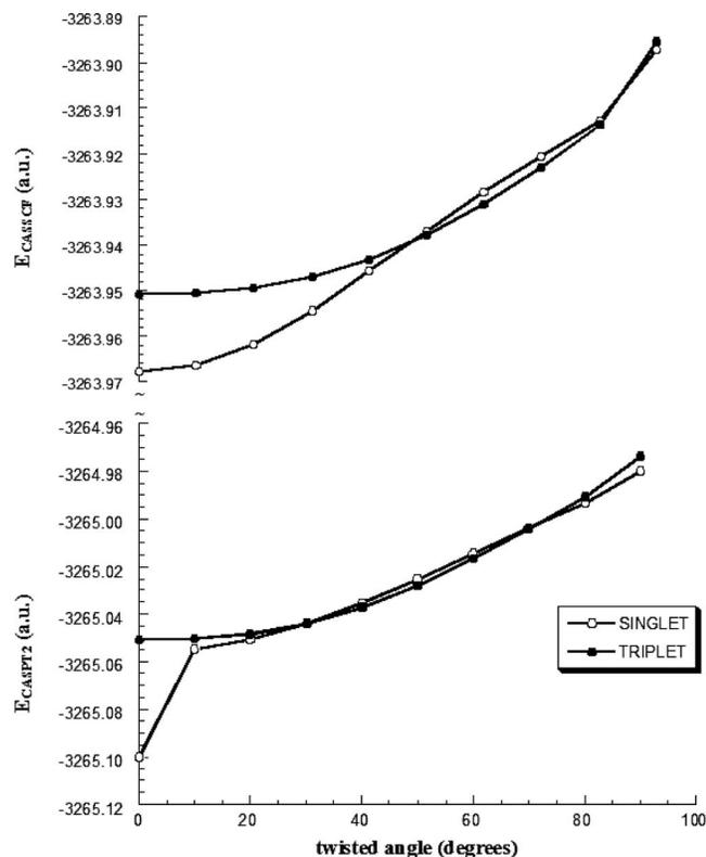
FIG. 4. The CASSF and CASPT2 energies of  $\text{Ni}(\text{S}_2\text{C}_2\text{H}_2)_2$  as a function of the twist angle. The moiety  $\text{S}_2\text{C}_2\text{H}_2$  is rotated around the  $z$  axis (Fig. 1).
