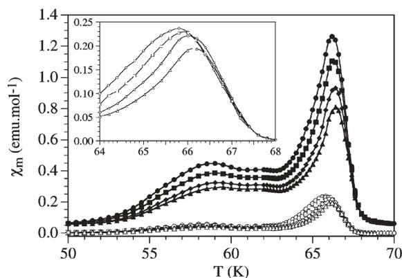
**Fig. 6** Frequency dependence of the AC susceptibility of **1** at 1, 10, 110 and 332 Hz (circles, squares, rhombuses and triangles, respectively).  $\chi'$  filled symbols,  $\chi''$  empty symbols. Inset shows the frequency dependence of the  $\chi''$  peak at ca. 66 K.
