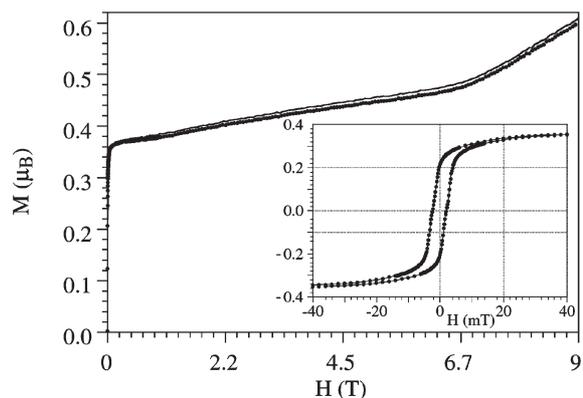
**Fig. 5** Isothermal magnetization at 5 K of **1**. Inset shows the hysteresis cycle and the rapid saturation in the low field region.
