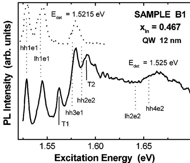
FIG. 7. PLE spectra at 2 K of the 12 nm thick QW of sample B1 ( $x_{\text{In}} = 0.467$ ) under two different detection energies (indicated in the figure). The possible optical transitions for this QW are indicated by dotted lines; they have been calculated as indicated below for  $Q_c = 0.13$ .
