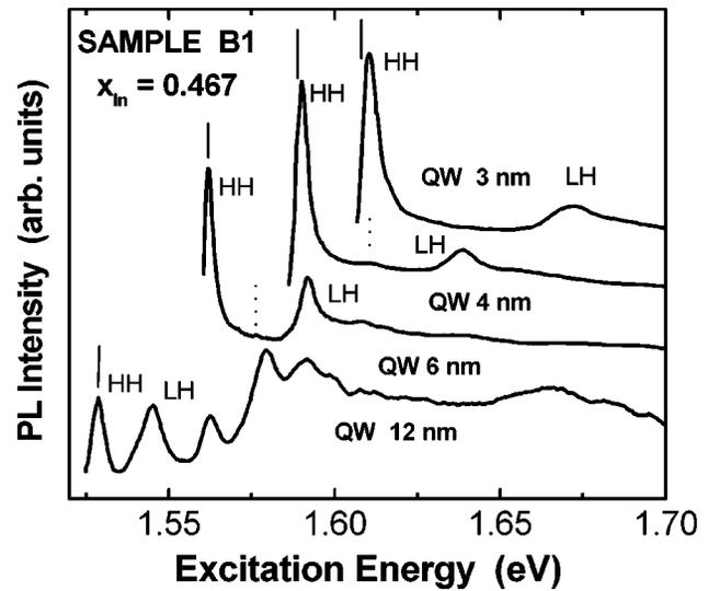
FIG. 6. PLE spectra at 2 K of the different QWs in sample B1 (near lattice matched to GaAs,  $x_{\text{In}}=0.467$ ). Short solid lines indicate the position of the PL peak energy (from Fig. 5) and short dotted lines the tentative position of the HH–exciton continuum onset. The detection energies for these spectra are 1.525, 1.561, 1.586, and 1.606 eV, corresponding to the 12, 6, 4, and 3 nm wide QWs, respectively.
