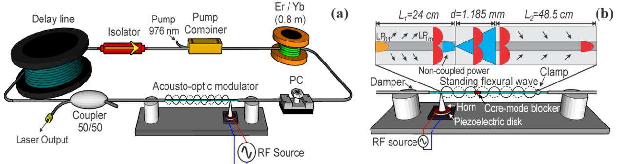
Figure 1. (a) Schematic setup of the mode-locked fiber ring laser. (b) Acousto-optic modulator.
