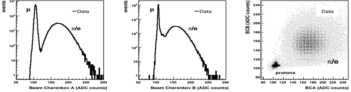
**Fig. 2.** Beam Cherenkov pulse height distributions. BCA in the left panel, BCB in the middle, and BCB vs. BCA in the right panel. The electron and pion tagging efficiency is found to be close to 100%; the peaks are separated by  $\approx 3\sigma$  in both detectors. By requiring a value compatible with a pedestal in both Cherenkov detectors the beam protons are clearly separable from pions and electrons as seen in the right panel.
