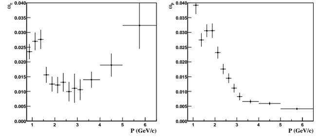
**Fig. 13.** Pion (left) and proton (right)  $\beta$ -outlier rates as a function of momentum. The pion outlier rate has been measured from the data; the proton outlier rate is estimated using the Monte Carlo. In reference [11] it has been demonstrated that no bias is seen when using the Monte Carlo to calculate the outlier rate.
