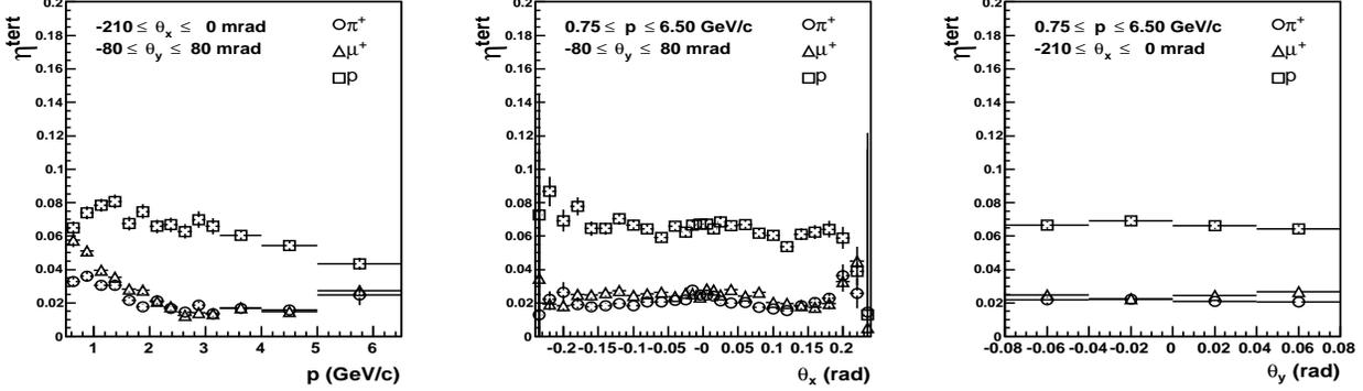
**Fig. 6.** Tertiary particle rates for pions, muons (which get identified as pions) and protons according to Monte Carlo simulation as a function of particle momentum (left), production angle in the horizontal plane,  $\theta_x$  (center) and production angle in the vertical plane,  $\theta_y$  (right).
