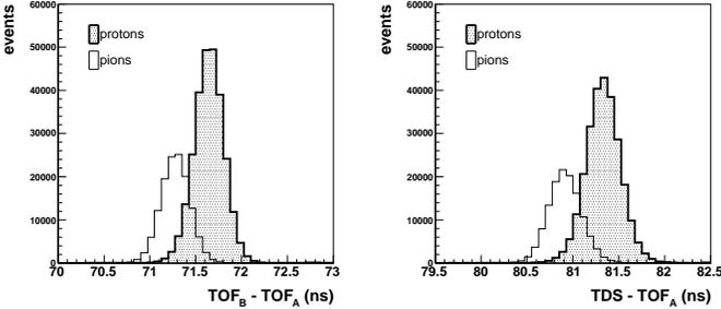
**Fig. 3.** Beam time-of-flight distributions. The time difference between TOFA and TOFB is shown in the left panel. The right panel is the time difference between TOFA and the TDS. The shaded distributions are for particles identified as protons by the Cherenkov detectors as described in the text. The open histograms are all other beam tracks: pions, electrons and muons from pion decays.
