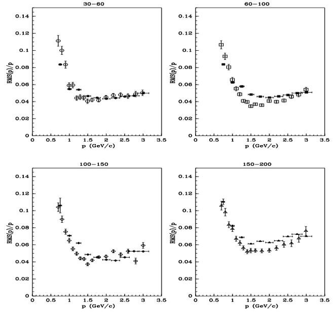
**Fig. 9.** RMS momentum resolution as a function of momentum in four angular bins (circles: 30 mrad–60 mrad; boxes: 60 mrad–100 mrad; diamonds: 100 mrad–150 mrad; triangles: 150 mrad–200 mrad). Data are shown with open symbols; Monte Carlo with filled symbols.
