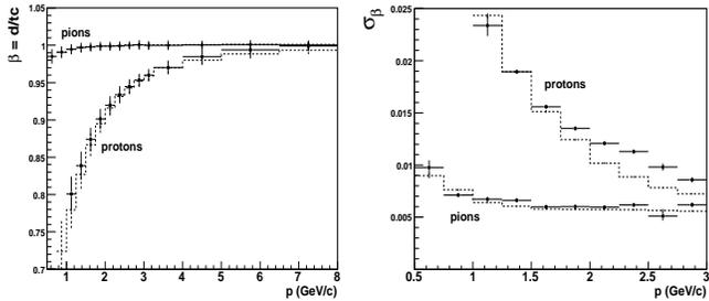
**Fig. 12.**  $\beta$  response for pions and protons as measured from data and Monte Carlo. The left panel shows the mean beta values with the error bars representing the width of the Gaussian distribution. The right panel highlights the width of the distributions and shows how the resolution asymptotically approaches  $\approx 0.006$ . The solid points are the response as measured from data; the dashed histograms are the response as measured from Monte Carlo.
