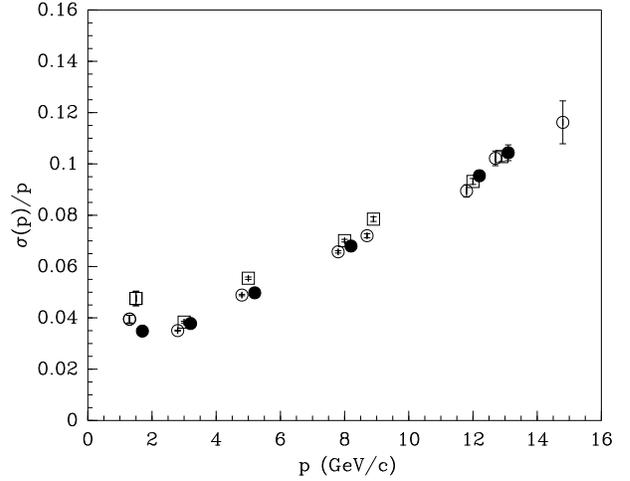
**Fig. 7.** Momentum resolution  $\sigma(p)/p$  (Gaussian fit) as a function of momentum (in GeV/c) for the drift chambers: the data were taken using several well-defined discrete beam momenta and no target for pions (open circles) and protons (open squares). Also shown (filled circles) is the corresponding resolution found using the Monte Carlo simulation.
