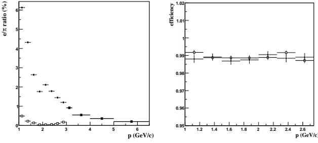
**Fig. 14.** The left panel shows the  $e/\pi$  ratio from a Monte Carlo simulation before (solid points) and after (open squares) the application of a 15 photo-electron cut. This cut reduces the electron contamination to 0.5% or less in the region where it is applied. The right panel shows the efficiency for pions (solid points) and protons (open squares) to pass the 15 photo-electron cut below 3 GeV/c, and is  $\approx 99\%$  for both.
