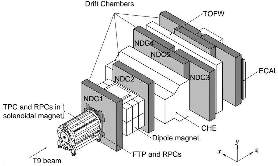
**Fig. 1.** Schematic layout of the HARP spectrometer. The convention for the coordinate system is shown in the lower-right corner. The three most downstream (unlabeled) drift chamber modules are only partly equipped with electronics and not used for tracking.
