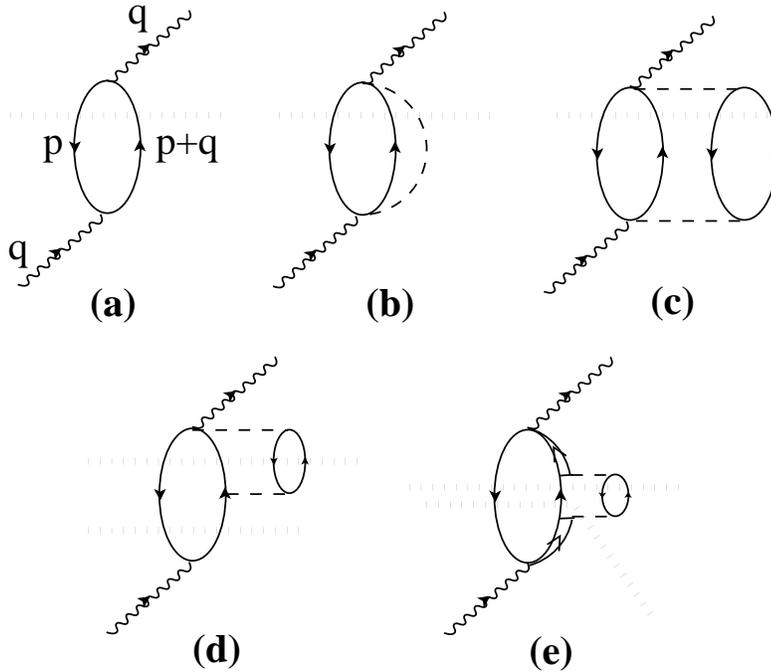
**Fig.1** Some many body Feynman diagrams whose imaginary parts contribute to the total inclusive ( $e, e'X$ ) cross section. The dotted lines indicate which particles are put on shell when evaluating the imaginary part of each diagram.
